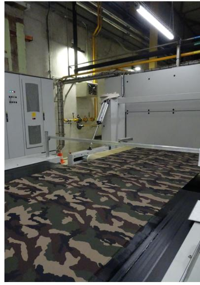
The printed fabric then goes through drying chambers before being stored in rolls, pending further processes.
